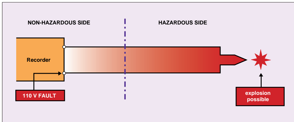
Figure 6. Thermocouple with fault
